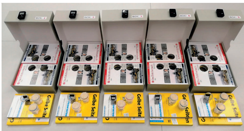
Figure 3 Five archival boxes prepared for the experiment, filled with telephone directories and four milled round recesses per box (© Judith Wagner).
