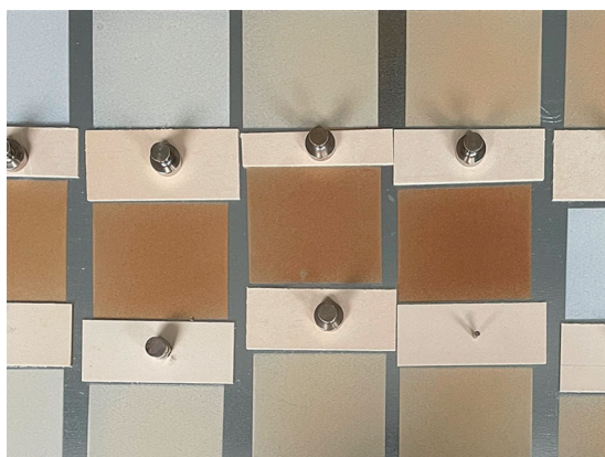
Figure 2. The fibre sheets at different toasting levels fixed on a metal plate with magnets. Bright brown, narrow blotter paper strips are placed beneath the magnets to ensure the films remain flat while drying on the metal plates (Photo: Lilian Samland).
