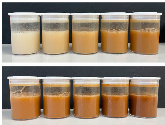
Figure 1. The fibre suspensions of the cellulose powder toasted at 200°C with increasing duration of thermal exposure (from left to right) (Photos: Lilian Samland).
