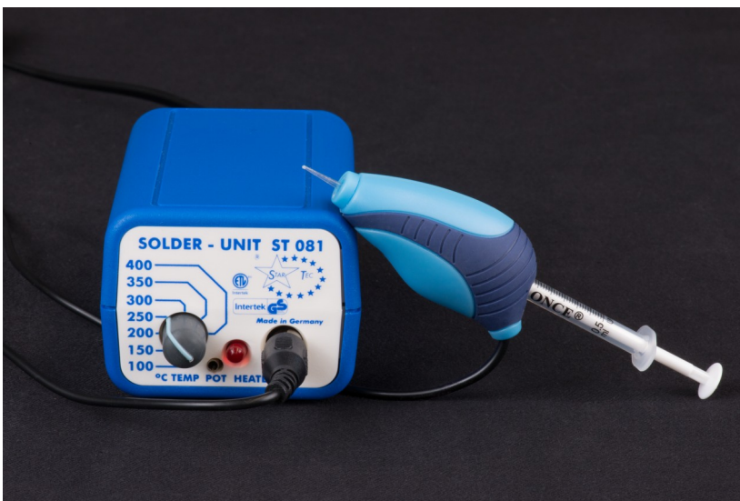
Fig. 3: Consolidation Pen „Winnie“: The heatable adhesive applicator and its control unit for temperature regulation. (Photo: Petra Demuth, 2019)
