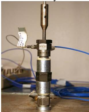
Figure 8: Hexagonal elastomer element & test setup
