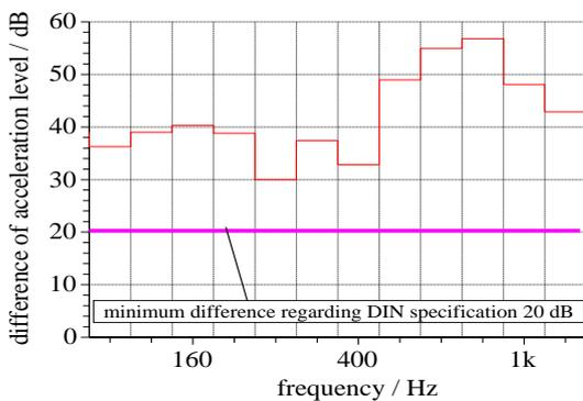
Figure 16: Ring-shaped elastomer element, frequency criterion, axial excitation
