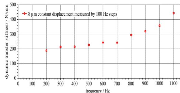
Figure 13: Ring-shaped elastomer element, dynamic transfer stiffness, radial excitation
