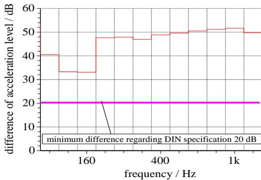
Figure 15: Ring-shaped elastomer element, frequency criterion, radial excitation
