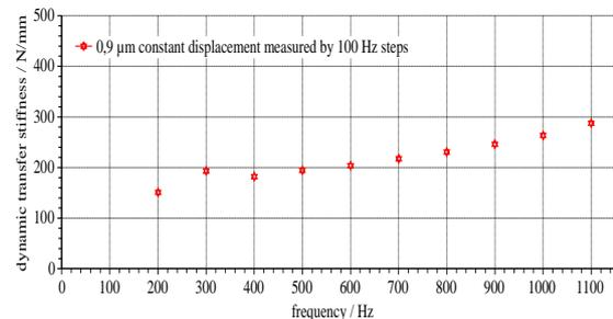
Figure 14: Ring-shaped elastomer element, dynamic transfer stiffness, axial excitation
