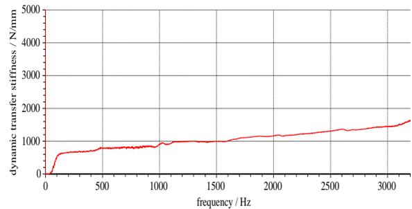
Figure 9: Dynamic stiffness of hexagonal elastomer element
