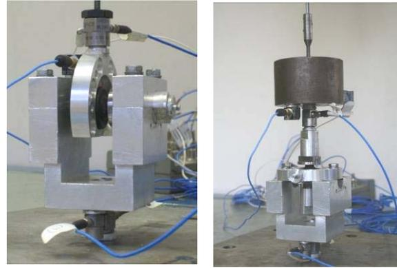
Figure 11&12: Ring-shaped element radial/axial test setup
