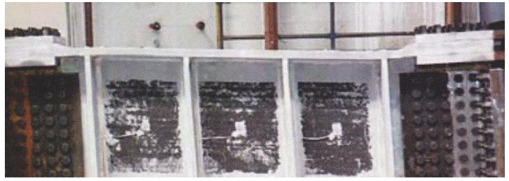
Full scale test of a shear link used in the tower
