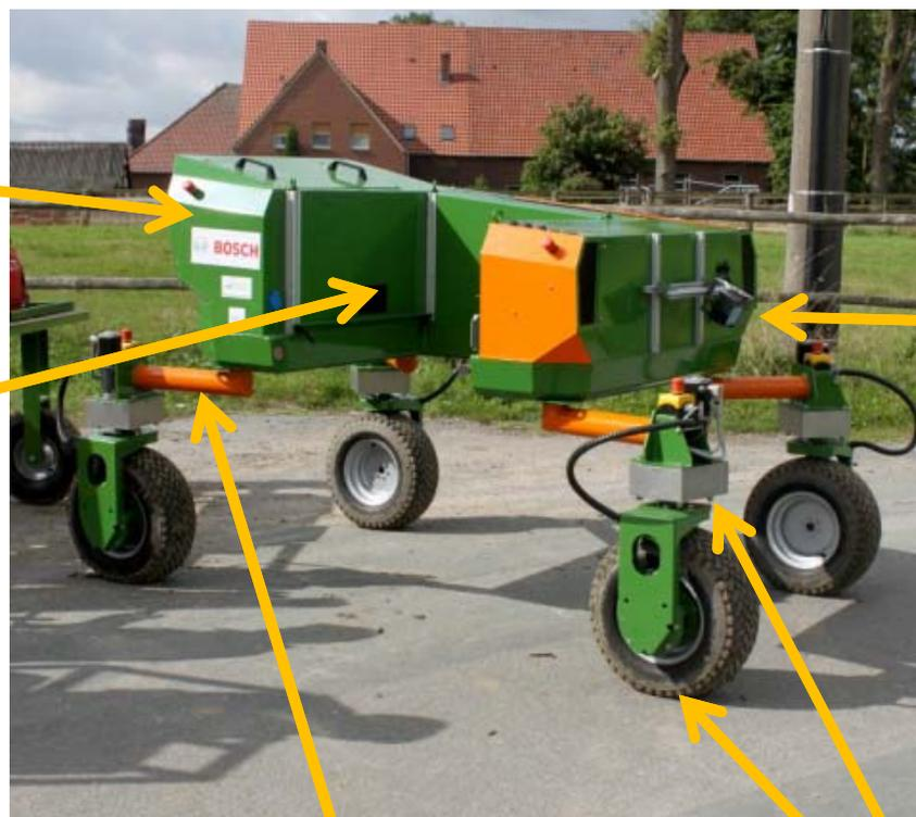
3D sensing for autonomous navigation (optionally navigation based on GPS)
