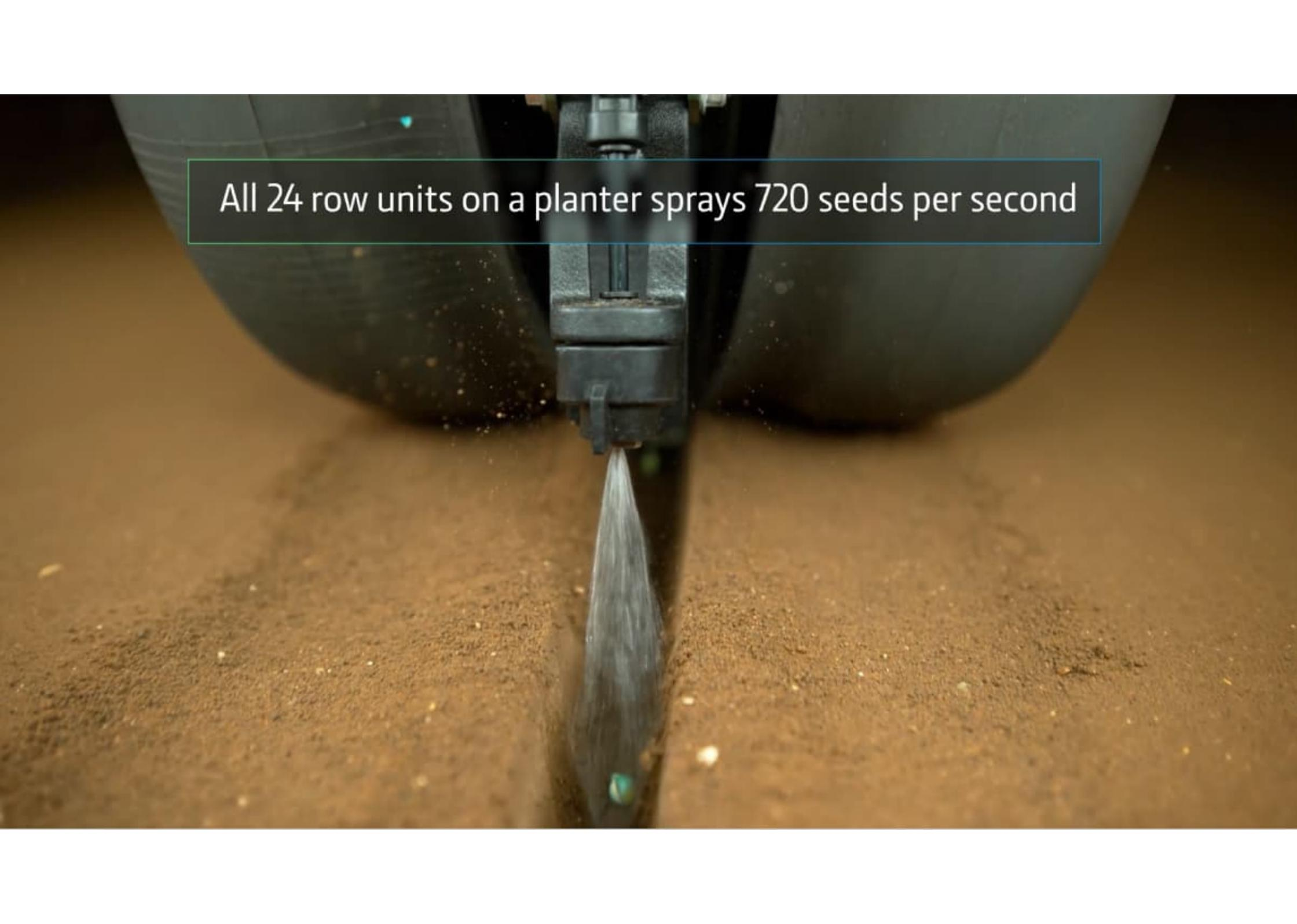
A close-up, low-angle shot of a planter's seed head. The central component is a dark, metallic-looking nozzle assembly. From the bottom of this assembly, a fine, mist-like spray of seeds is being emitted, falling into a narrow furrow in the brown soil. The surrounding soil is slightly blurred, emphasizing the precision of the seeding process. A semi-transparent text box is overlaid on the upper portion of the image.
