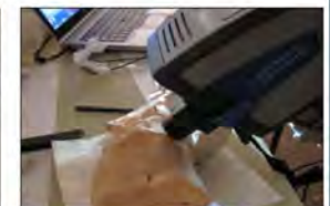
Non-invasive in-situ analysis of Umm al-Biyara polychrome fragment using a handheld FTIR and a USB microscope, PAP © Na'es 2017
